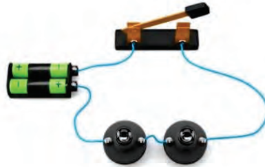
Fig 1.2.5: Connection of lamp in series
