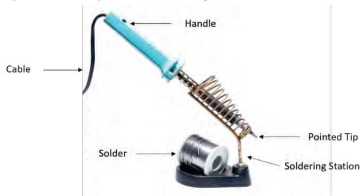
Fig 1.3.3: Parts of soldering iron
