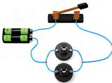
Fig 1.2.6: Connection of lamp in parallel
